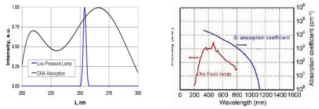
Flash lamps usually have length from ca. 10cm to 50cm, plus have also spiral or an arch and emit hundreds times as much in germicidal power as to compare to low pressure continuous wave UV (CWUV) lamps. It has strong advanatges for a number of applications where very hight degree sterilization is required (up to 6 logs, or ABSOLUTE) sterilization including UV and thermal resistant spores!
